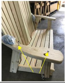
Fasten arms to arm rest supports by threading two 3" lags into the pre-drilled holes.
