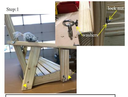
Place the seat in this position and fasten legs to seat assembly using two 2 1/4" bolts and the eye bolt.
