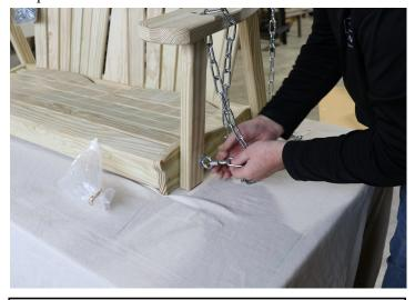
Fasten to quick link on the eye bolt. Use the other end to hang your swing at the desired location. On most applications, the angle of the swing will be correct, but it can be adjusted using either quick link. Repeat on opposite side.
