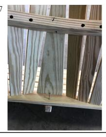
Fasten center seat support to bottom of backrest using screw provided.
