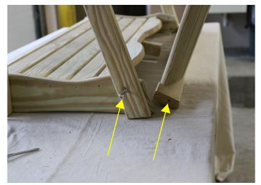
Thread a 3 1/2" lag into pre-drilled hole. Then align with pilot hole on backrest. Tighten after both sides are started.
