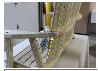
Fasten armrest to back support. On a 3" lag place a washer then the last link on the chain pack. Thread through pre-drilled hole on armrest into pilot hole on backrest. Overtightening can strip out the hole. If this happens, use a 4" lag(not provided). Repeat on opposite side.
