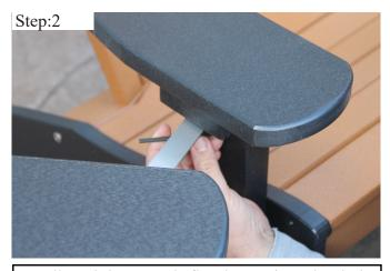
Install stainless steel flat bar using the bolts removed in step 1. This will create a wedge for the front part of the tete-a-tete to fit into.
