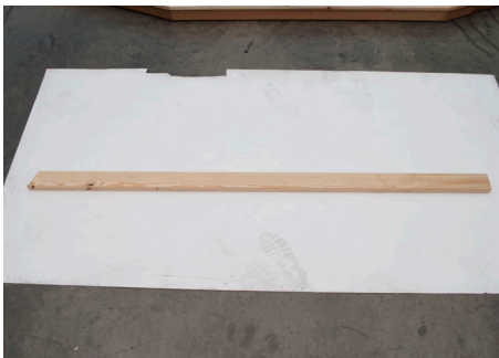
(2) Rafters Without Pre-Drilled Holes
